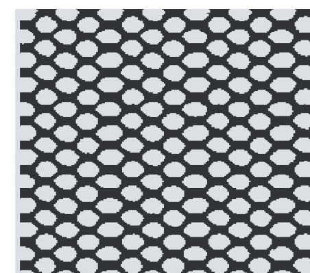
3. SCREEN - PERFORATED PANEL Manufacturer: Span MBS Material: Aluminum Profile: 27% Open Area Finish: Powder Coated Aluminum Color: SW 7646 "First Star"
